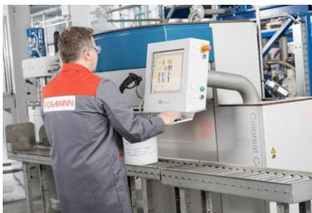
The highly user-friendly and extremely low-maintenance unit enables quick and economical production of even very small amounts of ink for individual use, for example 10-200 kg of one colour. The latest software supports the entire data management and recipes are stored in a database.
